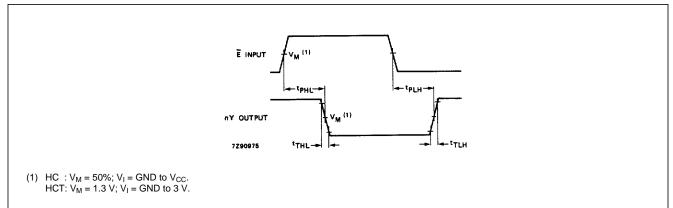
Fig.6 Waveforms showing the enable input  $(\overline{E})$  to output (nY) propagation delays and the output transition times.
